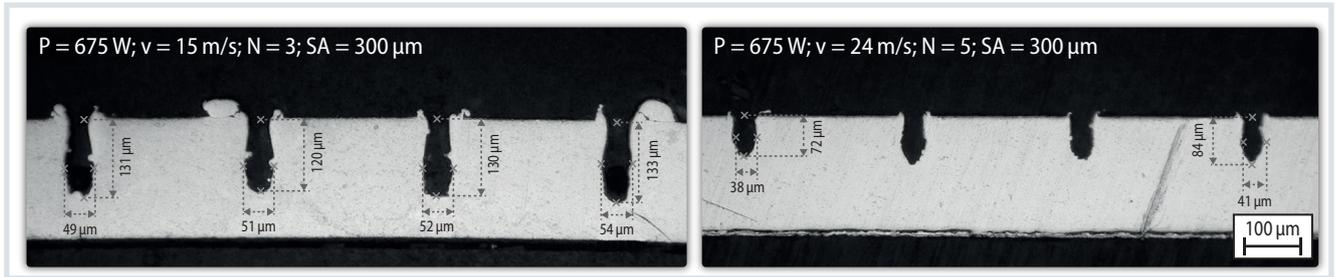
**Fig. 2.** Optimization of the structure geometry for thin aluminum sheet: through the scanning velocity and the number of passages, the geometry of the structure is adjusted. © Fraunhofer ILT
