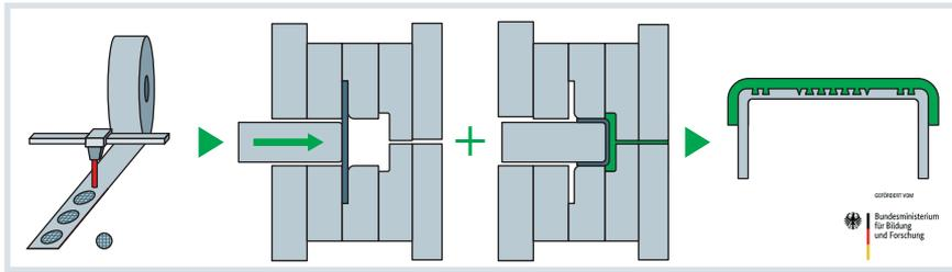
**Fig. 1.** Process for the production of mechanically interlocking plastic/aluminum crimp caps: cutting out and structuring of the thin metal sheet, insertion into the mold, forming, backmolding. Source: IKV; graphics: © Hanser
