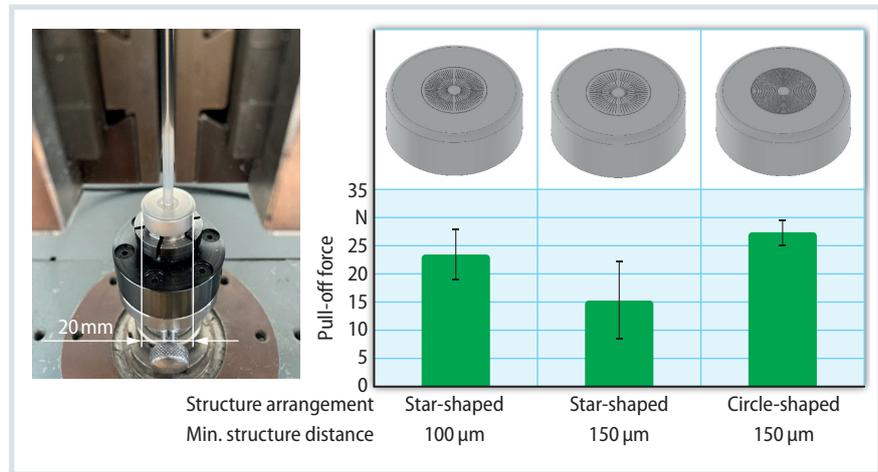
**Fig. 4.** Testing the bond strength in a vertical draw-off test (left). Result (right): the vertical draw-off force of the plastic component depends on the structural configuration. Source: IKV; graphics:
