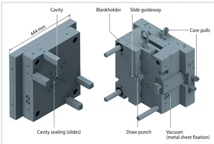
**Fig. 3.** Mold concept for the combined deep-drawing and backmolding process. Source: Hofmann; graphics: © Hanser
